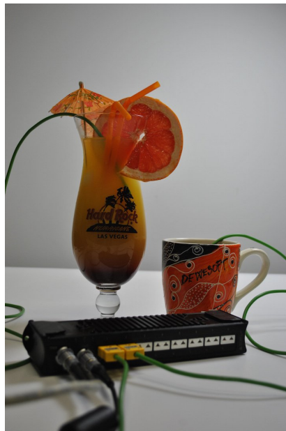
Image 29: One thermocouple immersed in a cold cocktail and the second one in a hot cup of tea
