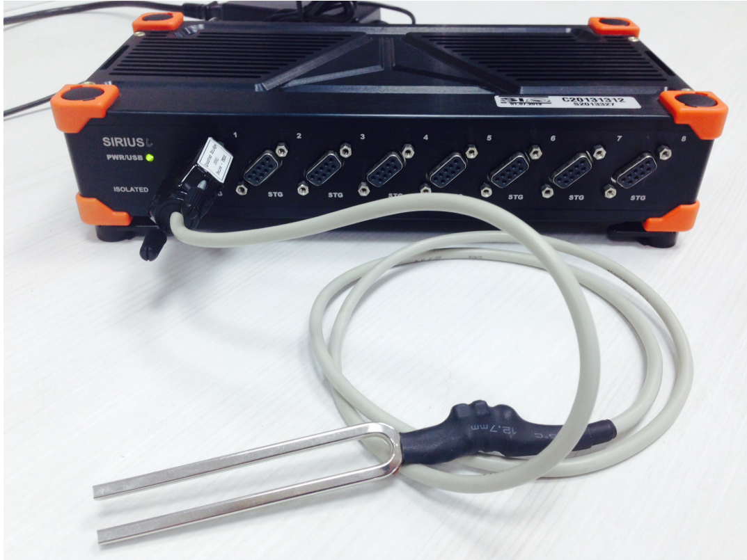
Image 25: Tuning fork connected to SIRIUS measurement system
