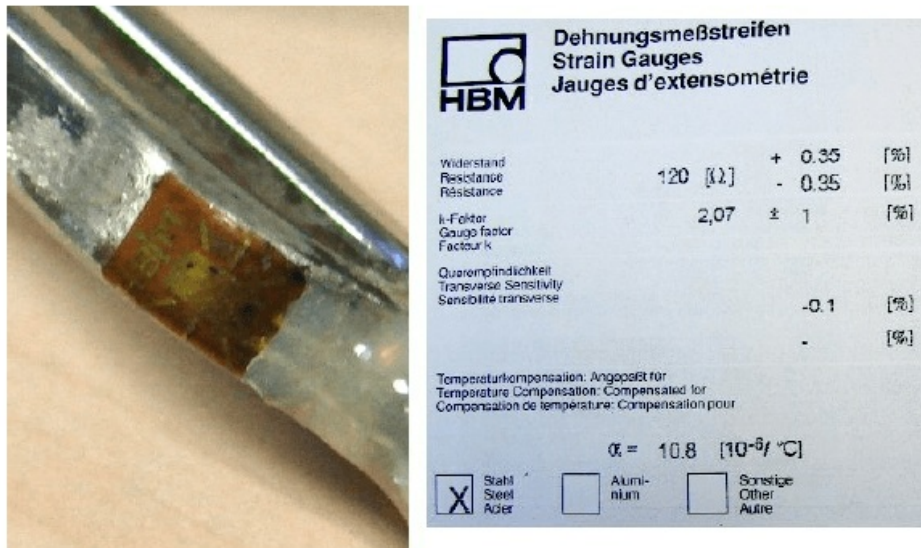
Image 26: Specifications of a strain gage
