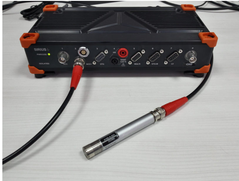
Image 21: Condenser microphone connected to SIRIUS DAQ device
