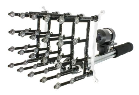
The CAE Intensity Array is an one dimensional sound intensity measurement system that is able to detect the source of very low frequencies. The output of the analysis is the sound intensity for each probe mapped on a picture. This measurement system is able to map stationary as well as transient noise sources.
