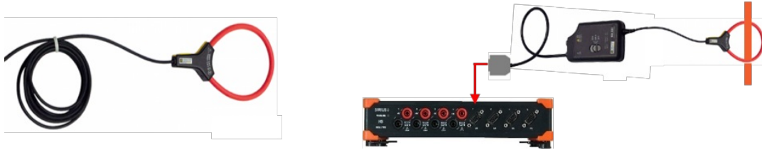
Image 3: Rogowski coil connected to a Sirius DAQ
