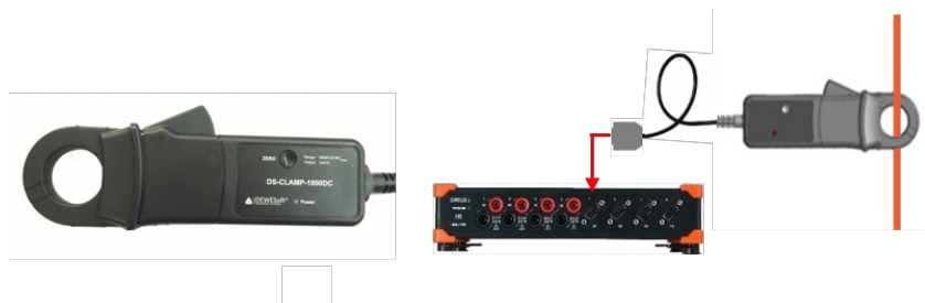
Image 7: Hall compensated clamp connected to a Sirius DAQ
