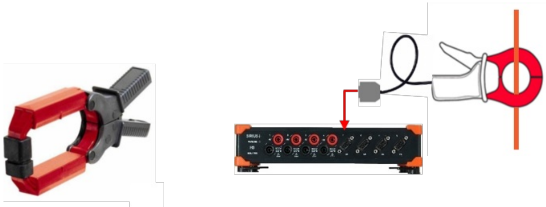
Image 5: Iron core clamp connected to a Sirius DAQ
