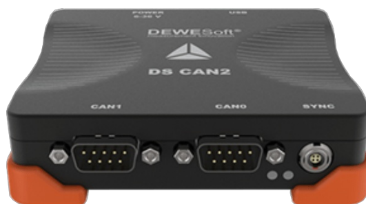
Image 10: DS-CAN2 is a 2xCAN port USB CAN interface device
