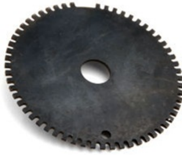
Image 5: Gear tooth with missing teeth
