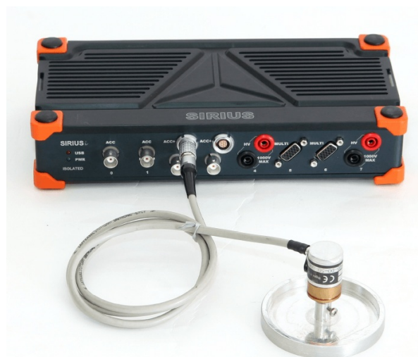
Image 4: Encoder connected to Dewesoft Sirius device
